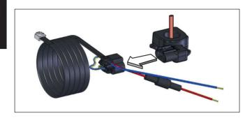
Please now connect the two power supply cables at the socket of the data cable with the battery terminals. Red cable on plus and blue cable on minus terminal of the battery.
